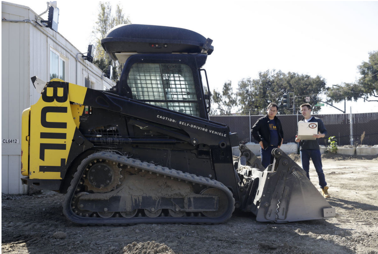
Bichen Wu, center, and Ed Walker use a laptop to determine what an autonomous bulldozer is seeing at Built Robotics Wednesday, Feb. 21, 2018, in San Francisco. Backed by Silicon Valley money, tech startups are developing self-driving bulldozers, drones to inspect work sites and robot bricklayers that can lay bricks faster than human and work without lunch breaks. (AP Photo/Marcio Jose Sanchez)
